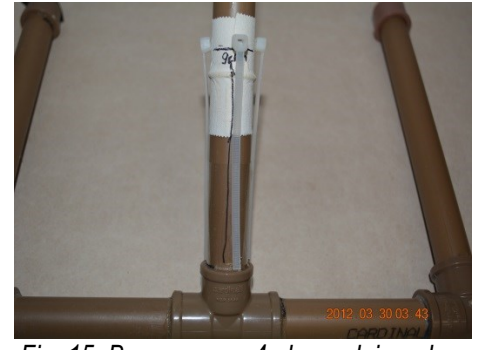
Fig. 15. Base com as 4 abraçadeiras de nylon.
