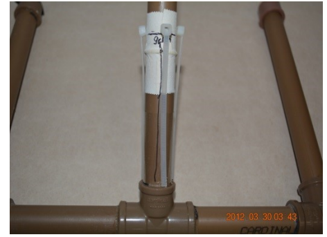
Fig. 15. Base com as 4 abraçadeiras de nylon.
