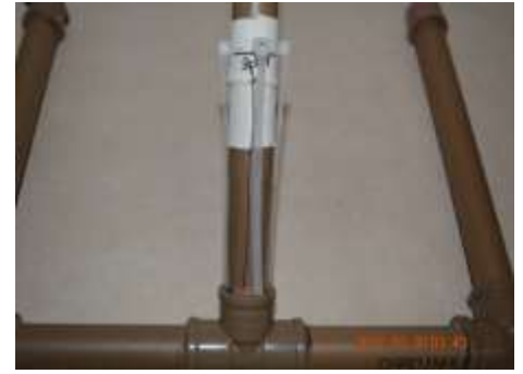
Fig. 15. Base com as 4 abraçadeiras de nylon.
