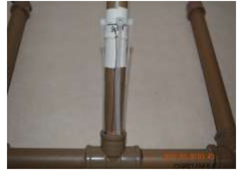
Fig. 15. Base com as 4 abraçadeiras de nylon.
