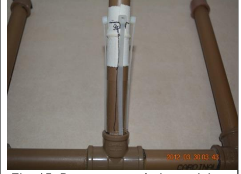
Fig. 15. Base com as 4 abraçadeiras de nylon.
